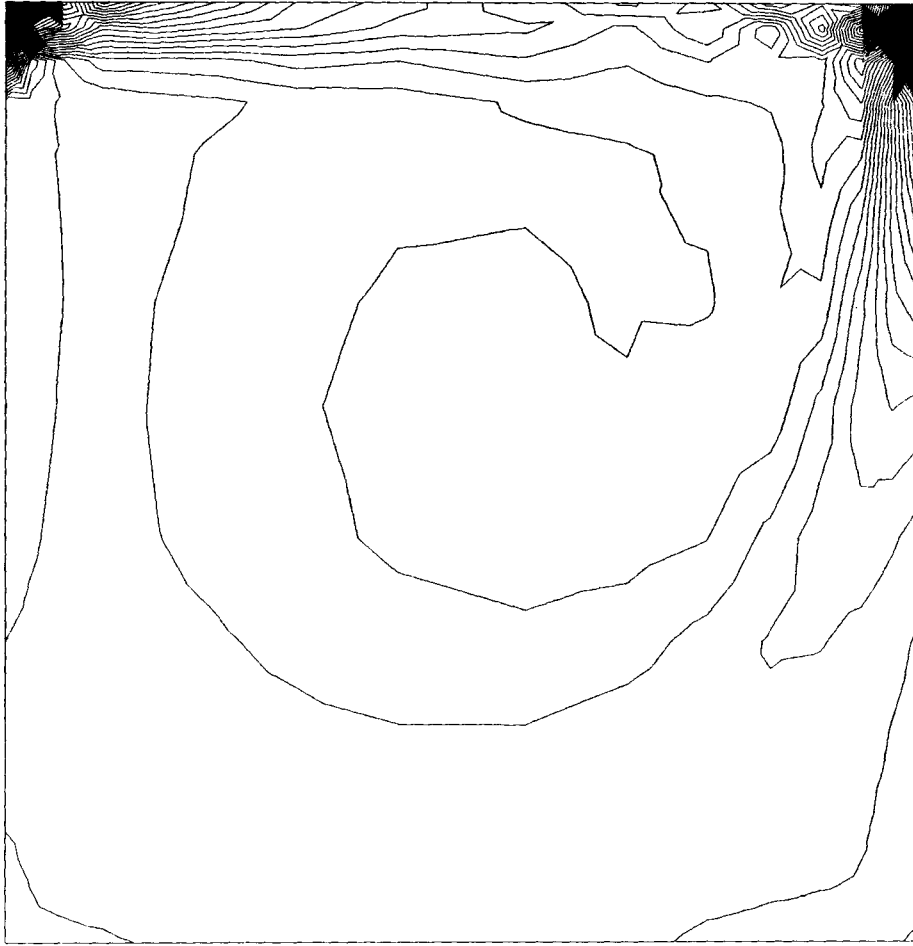
Figure 3(b). Equivorticity lines for driven cavity, streamfunction-vorticity, Re = 400
